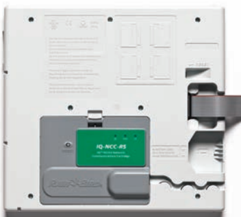
RS -232 CARTRIDGE INSTALLED IN ESP-LX
