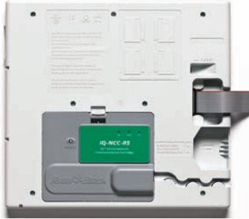
RS-232 CARTRIDGE INSTALLED IN ESP-LX
