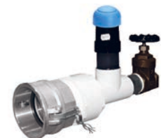
Header Air Release/Flush Out: Pre-assembled with Female Cam, 2" Gate Valve, PVC Fittings & Relief Vent.
