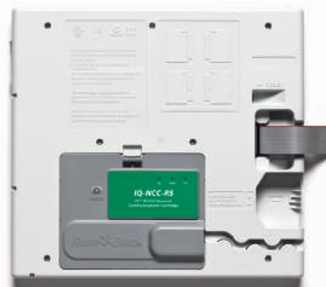
RS -232 CARTRIDGE INSTALLED IN ESP-LX
