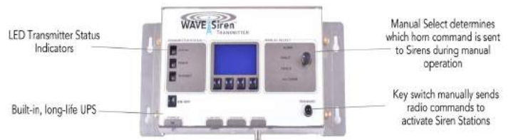
LCD Display and multi-purpose navigational buttons allow users to view the Transmitter status, configuration and user menus.
